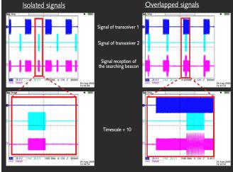
The overlapping of signals is the major source of problems during close multiple burial situati-ons. The transmitting strategy chosen by the beacon manufacturer is an issue of fundamental importance here, due to the fact that an overlapped signal can no longer be isolated, not even with digital signal processing.
