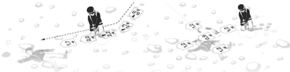
**Important!** Before the direction arrows are suppressed, the last distance correction has to be done exactly. You are then moving to the transmitting beacon in best coupling position and save time during the cross-like movements. In the case of a deep burial it could happen that the minimum direction indication is higher than 2 m!
