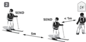
**TIP!** The receive control can be combined with a range test in long distance.
