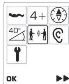
If the S1 receives an audible (via the loudspeaker) and visible signal (circle with 2 persons) from each individual avalanche transceiver then the transmission function of the units to be tested and the reception function of the group leader are in order.
