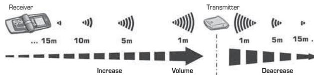
The ORTOVOX safety emergency reception allows an acoustic search even when the batteries have almost completely run out. When a battery change has been delayed (remaining capacity less than 10 %), sensors and display are automatically switched off, as the minimum current supply is no longer reached. Now only an acoustic reception is available.
