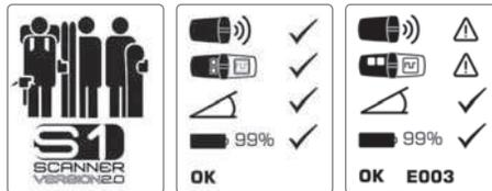
*If an error function or fault is detected, the warning triangle appears.*
