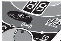
If two signals of approximately the same strength are received, then the direction arrows flash alternately. The red LED is illuminated. In this case the searcher will decide which of the two directions he will follow.
