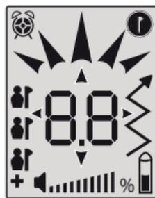
The device then displays the software version installed and remaining battery life. We recommend that you replace the batteries as soon as it drops below 50%. Holding down the marking button in transmit mode will allow you to check battery life left at any time.
