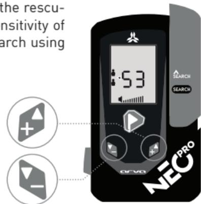
The left and right arrows blink in turn to help the rescuer calibrate the sensitivity correctly.
