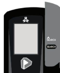
3. Turn on the device while keeping the marking button pressed down until the first setting to appears: the automatic revert-to-transmit time without movement (the number "4" blinks on screen).
