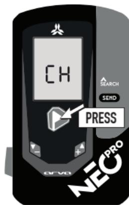
You will then be able to test your partners' devices one by one by positioning your device 1m away from each device you check. It is important to remain 1m away from each device for the GROUP CHECK to work properly, otherwise your device will start "double beeping" to indicate that you are too close or too far away.
