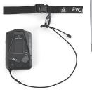
Position the EV05 in a zippered pant pocket for the entire duration of your outing. The zipper slider should be fully closed, leaving only enough room for the elastic cord to exit. Adjust the belt around your waist and then buckle it.
