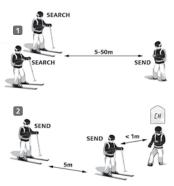
Press the main switch lock and push the main switch to the "SEND" position. The display indicates the SEND-symbol, the remaining battery capacity, and the transmitting antenna. Additionally an LED indicator light flashes simultaneous with the transmitter bit timing.
