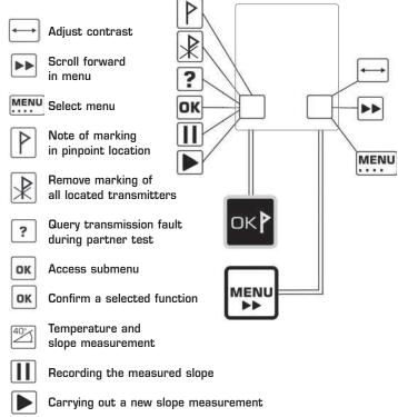
The S1 allows the temperature and the slope angle to be measured.
